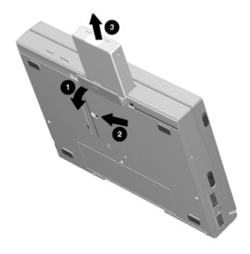
Figure 5-11. Removing the Hard Drive
